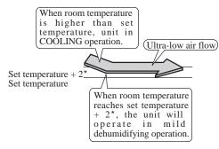
In Heating operation, after start the unit, the air conditioner will sending warm air a moment later to prevent the cold air blowing out. In Dehumidifying, when the room temperature drops 2\* higher than the set temperature, regardless the set fan speed, the air conditioner will intermittently operate in low fan speed.
